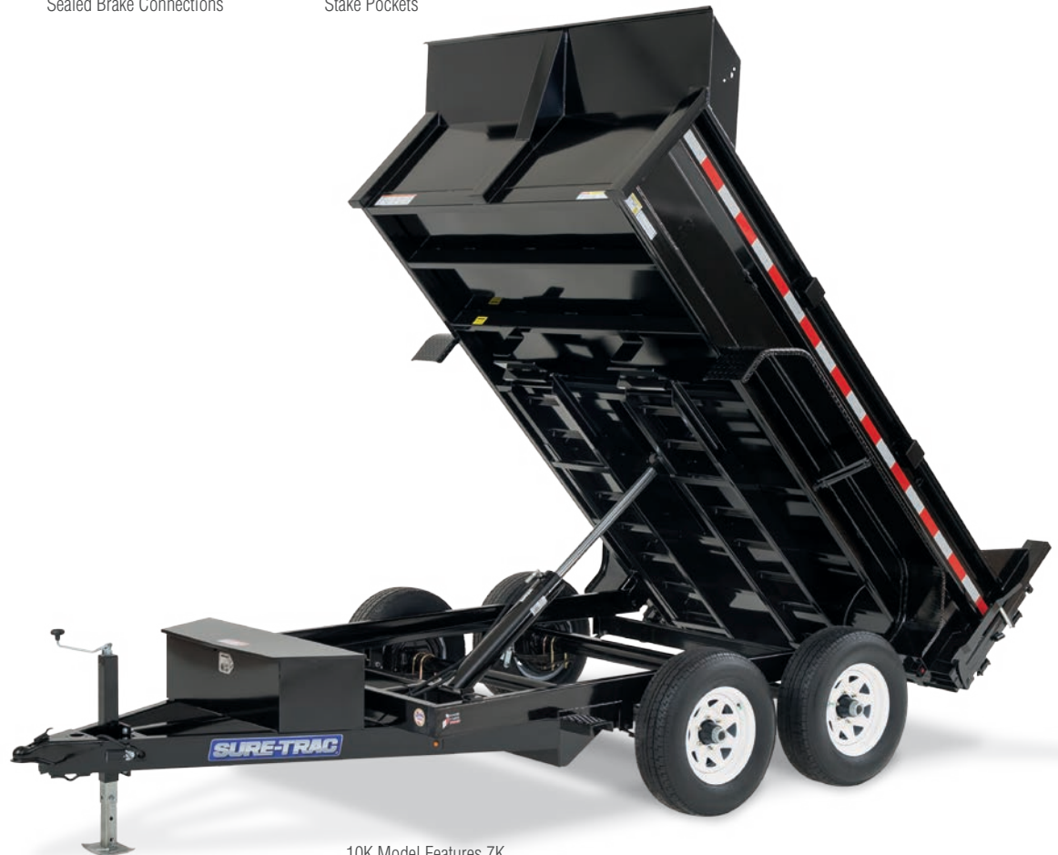
10K Model Features 7K Dropleg Jack, Ramps and Combo Gate
