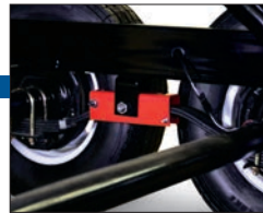
Slipper Spring Suspension - 14K and Up
